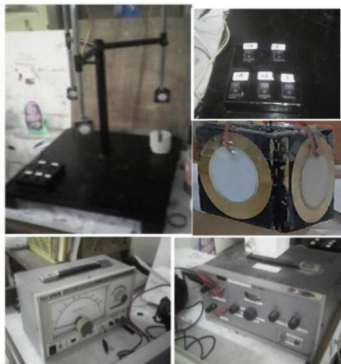
Figure 2. The Equipment Employed in this Study, viz.: the Sonicator System (top-left), Sonicator Control Panel (top-right), Csi/Speco Audio Generator Model SS-1 [20 Hz – 2 MHz] (bottom-left), Uchida Amplifier TA-2MS (bottom-right), and Piezoelectrics (Middle-Right)
