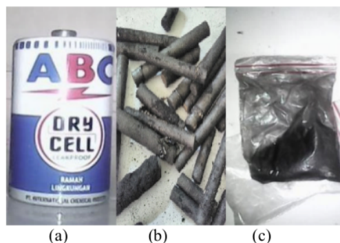
Figure 1. The Materials Treated in this Study: (a) a Used ZnC Battery; b) Carbon Rods from the Battery; and (c) Carbon Powder Obtained from the Carbon Rods
