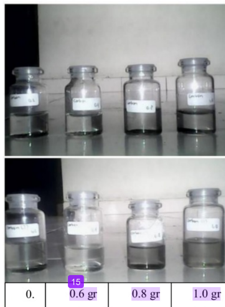
Figure 3. The Solutions with Powder Mass Variations before (top) and after (bottom) Sonications
